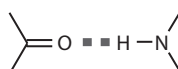
FIGURE 2.3 Hydrogen bonds. Hydrogen bonds (blue) form between electronegative acceptor groups (O) and electropositive donor groups (NH).
